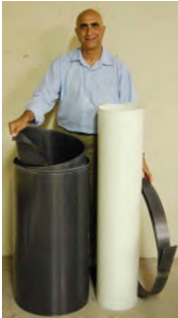
Fig. 1. From left to right: carbon and glass PileMedic® laminates and unidirectional carbon strips. Note the flexibility of PileMedic® being bent by hand.
