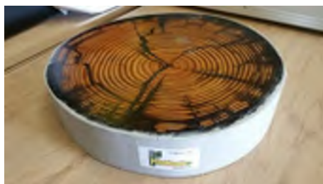
Fig. 2. Penetration of low viscosity resin into all cracks and voids
